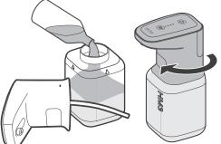
Pour alcohol into the bottle until the maximum level mark on the top back of the container, and then twist the lid to tighten it back to its original position. ※ Please keep the silicone pipe clean and dust-free before screwing the lid back onto the container
